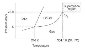
Fig. 1. Phase diagram of carbon dioxide (Ginty et al., 2005)
